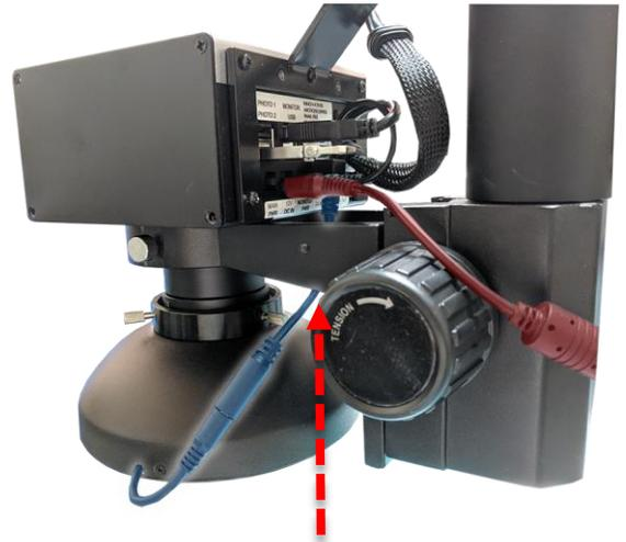
Connect the dome ring light pigtail through the focus mount as shown
